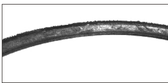
Shining surface due to high slippage
